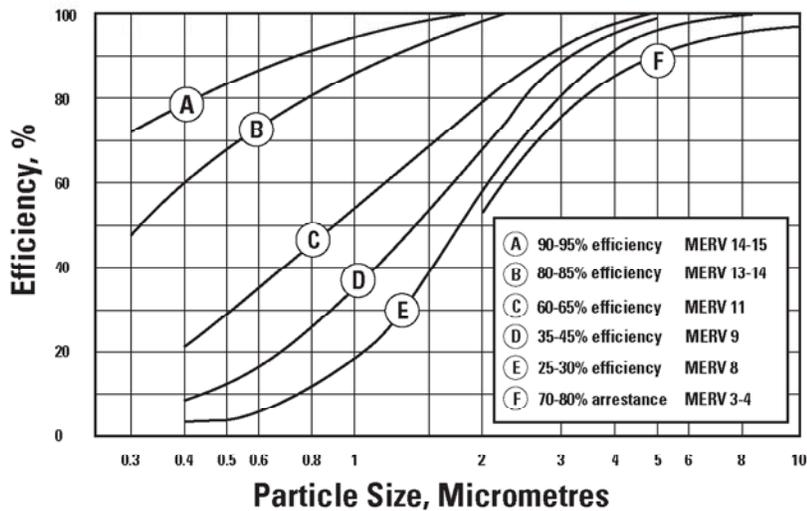
0.3 to 10 micron in size. This value is based on the lowest, or minimum efficiency for the filter. In many cases this is when the filter is first installed.
