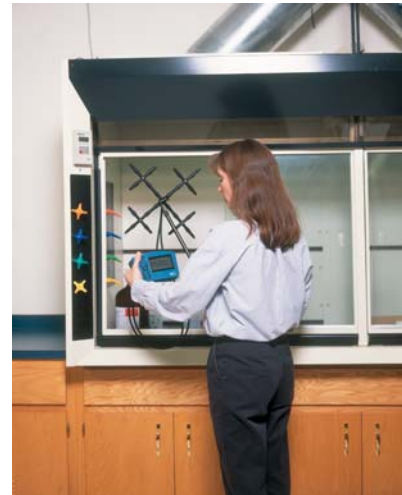
Figure 15. Face velocity is the primary method of evaluating fume hood performance after initial set-up.
