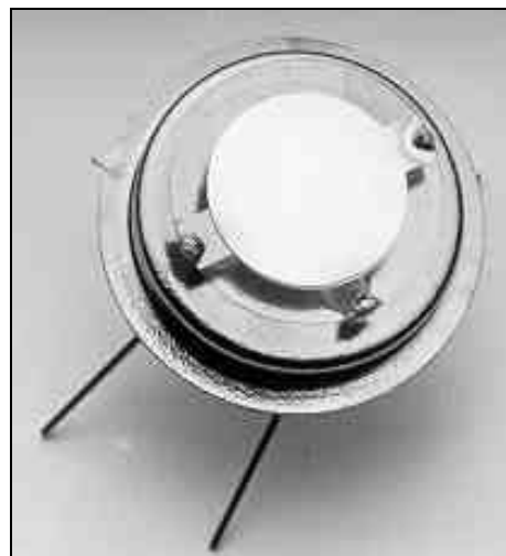
Figure 2 - Quartz crystal microbalance
